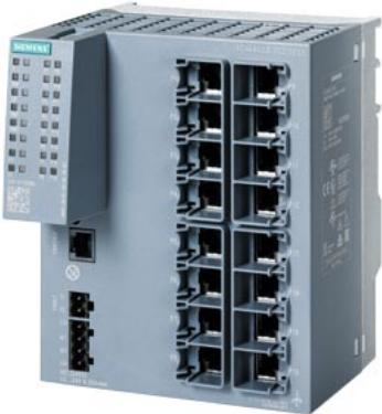
SCALANCE XC216EEC manageable Layer 2 IE switch; IEC 62443-4-2 certified; 16x 10/100 Mbit/s RJ45 ports; 1x console port; diagnostics LED; redundant power supply; with painted printed-circuit boards; NAMUR NE21-compliant; temperature range -40 °C to +70 °C; assembly: DIN rail/S7 mounting rail/wall redundancy functions; office features (RSTP, VLAN,...); PROFINET IO device; Ethernet/IP-compliant; C-PLUG slot;
