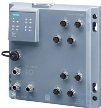
SCALANCE XP208PoE EEC, managed IE switch, 8x 10/100 Mbit/s IEC 62443-4-2 certified; M12 ports, IP65, LED diagnostics, error signaling contact, redundant power supply, PROFINET IO device, network management, can be operated in redundant ring, dust caps, including electronic manual on CD-ROM, C-plug optional.
