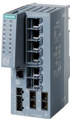
SCALANCE XC206-2 manageable Layer 2 IE switch; IEC 62443-4-2 certified; 6x 10/100 Mbit/s RJ45 ports; 2x 100 Mbit/s SC-ports, 1x console port; diagnostics LED; redundant power supply; temperature range -40 °C to +70 °C; assembly: DIN rail/S7 mounting rail/wall; redundancy functions; office features (RSTP, VLAN,...); PROFINET IO device Ethernet/IP-compliant C-PLUG slot.
