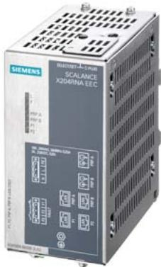
SCALANCE X204RNA EEC; redundant network access 2x 100 Mbit/s RJ45 ports; 2x 100 Mbit/s combo ports; LED diagnostics; error signaling contact with set pushbutton; simple power supply; network management; including electronic manual on CD-ROM, C-PLUG optional for HSR network;
