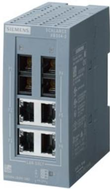
SCALANCE XB004-2 unmanaged Industrial Ethernet Switch for 10/100 Mbit/s; for setting up small star and line topologies; LED diagnostics, IP20, 24 V DC power supply, with 4x 10/100 Mbit/s twisted pair ports with RJ45 sockets; 2x 100 Mbit/s multimode glass fiber-optic cable port with SC socket; manual available as a download .
