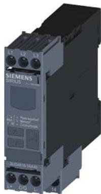
!!! product phase-out !!! the preferred successor is 3UG5816-1AA40 line monitoring IO-Link, 3x 160-690 V digital monitoring relay for 3-phase line voltage for IO-Link 50...60 Hz AC 3 x 160 to 690 V phase sequence, phase failure phase asymmetry undervoltage and overvoltage hysteresis 1-20 V line stabilization delay tripping delay time 1 changeover contact, screw terminal
