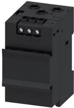
current/voltage measuring module for dry-running protection of centrifugal pumps in hazardous areas, current setting 0.3...4 A, voltage measurement up to 690 V, width 45 mm, straight-through transformer
