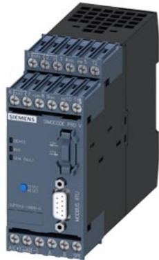
basic device SIMOCODE pro V MR, MODBUS RTU interface 57.6 Kbps, RS-485, 4 I/3 O freely configurable, Us: 24 V DC, input for thermistor connection monostable relay outputs, expandable by expansion modules
