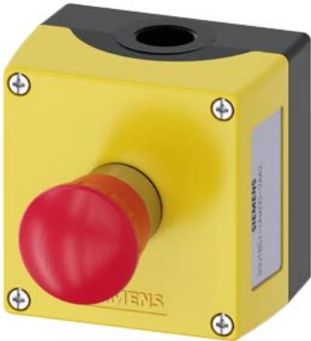
Enclosure for command devices, 22 mm, round, Enclosure material metal, Enclosure top part yellow, 1 control point metal, A=EMERGENCY STOP mushroom pushbutton red, 40 mm, rotate-to-unlatch, Control point in center, 1 NC, screw terminal, floor mounting, 1xM20 each on top and bottom
