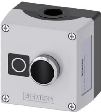
Enclosure for command devices, 22 mm, round, Enclosure material metal, enclosure top part gray, 1 control point metal, A=Pushbutton black, 1 NC, screw terminal, floor mounting, label: O, 1xM20 each on top and bottom, Label enclosed
