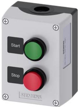
enclosure for command devices, 22 mm, round, enclosure material plastic, enclosure top part gray, 2 control points plastic, B=Pushbutton green, label: start, 1 NO, screw terminal, A=Pushbutton red, raised, label: Stop, 1 NC, screw terminal, floor mounting, 1xM20 each on top and bottom, Labels glued in
