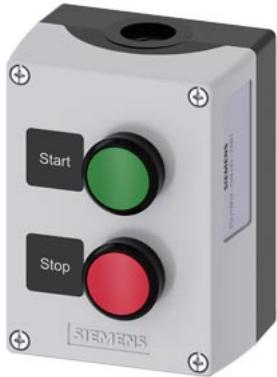
enclosure for command devices, 22 mm, round, enclosure material plastic, enclosure top part gray, 2 control points plastic, B=Pushbutton green, label: start, 1 NO, screw terminal, A=Pushbutton red, label: Stop, 1 NC, screw terminal, floor mounting, 1xM20 each on top and bottom, Labels glued in
