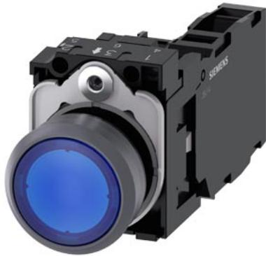
Illuminated pushbutton, 22 mm, round, plastic with metal front ring, blue, pushbutton, flat, momentary contact type, with holder, 1 NO+1 NC, LED module with integrated LED 230 V AC, screw terminal
