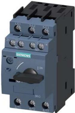
Circuit breaker size S0 for transformer protection A-release 16...22 A N-release 364 A screw terminal Standard switching capacity with transverse auxiliary switches 1 NO+1 NC
