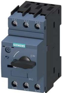
Circuit breaker size S00 for transformer protection A-release 0.7...1 A N-release 21 A screw terminal Standard switching capacity
