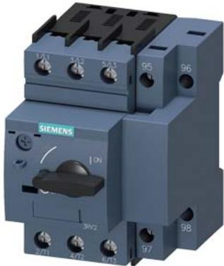
Circuit breaker size S00 for motor protection, CLASS 10 with overload relay function A-release 0.22...0.32 A N-release 4.2 A screw terminal Standard switching capacity
