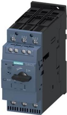
Circuit breaker size S2 for motor protection class 20 A-release 54...65 A N-release 845 A screw terminal Standard switching capacity with transverse auxiliary switches 1 NO+1 NC
