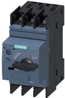
Circuit breaker size S00 for motor protection, CLASS 10 A-release 2.2...3.2 A N release 42 A ring cable lug connection Standard switching capacity
