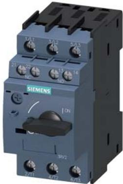
Circuit breaker size S00 for motor protection, CLASS 10 A-release 2.2...3.2 A N release 42 A screw terminal Standard switching capacity with transverse auxiliary switches 1 NO+1 NC
