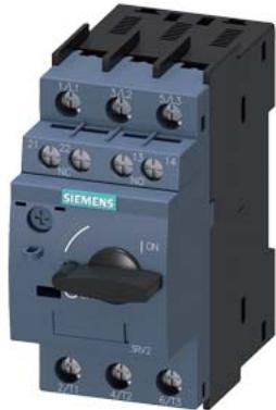
Special type Circuit breaker size S00 for motor protection, CLASS 10 A-release 1.8...2.5 A N-release 33 A screw terminal Standard switching capacity with transverse auxiliary switches 1 NO+1 NC Ambient temperature -50 °C 500 switching cycles
