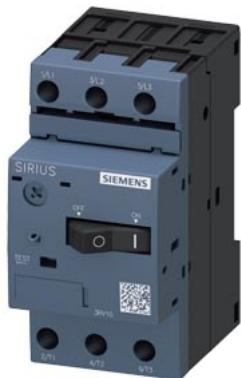
Circuit breaker size S00 for motor protection, CLASS 10 A-release 0.55...0.8 A N-release 10 A Screw terminal Standard switching capacity
