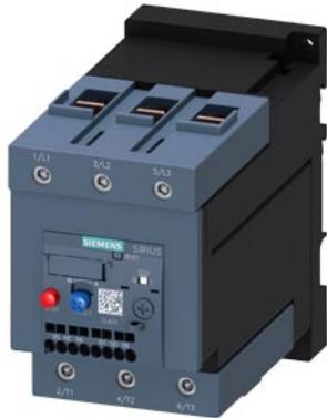
overload relay 80...100 A thermal for motor protection frame size S3, Class 10 stand-alone installation main circuit: screw auxiliary circuit: spring-loaded terminal manual-automatic RESET
