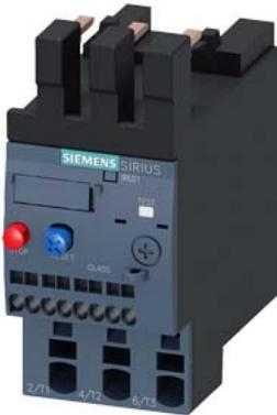
overload relay 30...36 A thermal for motor protection frame size S0, Class 10 for mounting on contactors main circuit: spring-loaded terminal auxiliary circuit: spring-loaded terminal manual-automatic RESET
