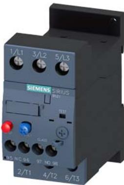
Overload relay 23...28 A Thermal For motor protection Size S0, Class 10 Stand-alone installation Main circuit: Screw Auxiliary circuit: Screw Manual-Automatic-Reset
