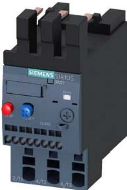
overload relay 11...16 A thermal for motor protection frame size S0, Class 10 for mounting on contactors main circuit: spring-loaded terminal auxiliary circuit: spring-loaded terminal manual-automatic RESET
