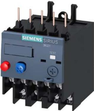
Overload relay 0.35...0.50 A Thermal For motor protection Size S00, Class 10
