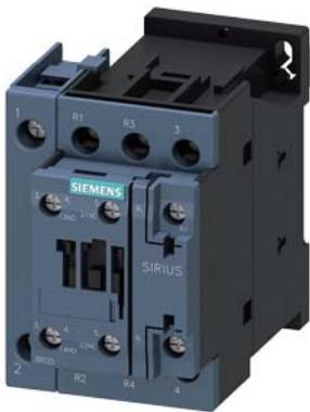
power contactor, AC-3, 25 A, 11 kW / 400 V, 4-pole, 110 V AC, 50 Hz / 120 V, 60 Hz, main contacts: 2 NO + 2 NC, auxiliary contacts: 1 NO + 1 NC, screw terminal, size: S0
