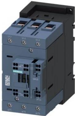
traction contactor, AC-3e/AC-3, 110 A, 55 kW / 400 V, 3-pole, 110 V DC, 0.7-1.25\* Uc, solid-state operating mechanism, with integrated varistor, auxiliary contacts: 1 NO + 1 NC, main circuit: screw terminal, control and auxiliary circuit: spring-loaded terminal, frame size: S3
