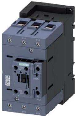
power contactor, AC-3e/AC-3, 110 A, 55 kW / 400 V, 3-pole, 20-33 V AC/DC, 50/60 Hz, with integrated varistor, auxiliary contacts: 1 NO + 1 NC, screw terminal, size: S3, communication-capable
