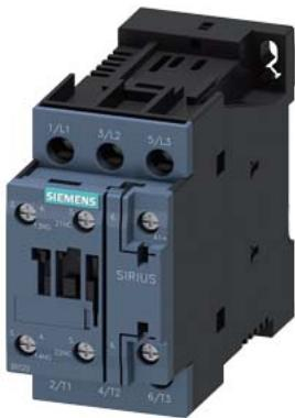
power contactor, AC-3e/AC-3, 25 A, 11 kW / 400 V, 3-pole, 24 V DC, auxiliary contacts: 1 NO + 1 NC, screw terminal, size: S0
