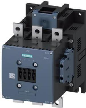
power contactor, AC-3e/AC-3 300 A, 160 kW / 400 V, AC (50-60 Hz) / DC Uc: 110-127 V 3-pole, auxiliary contacts 2 NO + 2 NC drive: conventional main circuit: busbar control and auxiliary circuit: screw terminal
