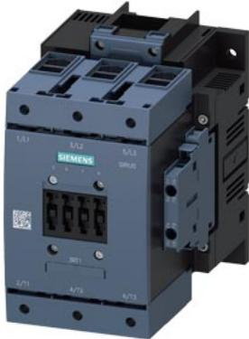
power contactor, AC-3e/AC-3 115 A, 55 kW / 400 V, AC (50-60 Hz) / DC Uc: 220-240 V 3-pole, auxiliary contacts 2 NO + 2 NC drive: conventional main circuit: box terminal control and auxiliary circuit: screw terminal
