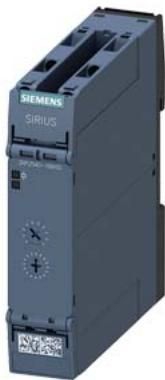
Timing relay, electronic OFF delay without control signal or smooth passing make contact non-volatile 7 time ranges 0.05...600 s 12-240 V AC/DC, 2 change-over contacts at 50/60 Hz AC with LED, Screw terminal
