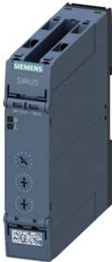
Timing relay, Multifunction 2 change-over contacts, 27 functions 7 time ranges (0.05 s...100 h) 24 V AC/DC at 50/60 Hz AC with LED, Screw terminal
