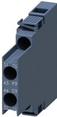
auxiliary switch, lateral, 1 NO + 1 NC, on the left: 51/52, 63/64, on the right: 31/32, 43/44, current path: 1 NC, 1 NO, screw terminal, for contactors 3RT2 and contactor relays 3RH2
