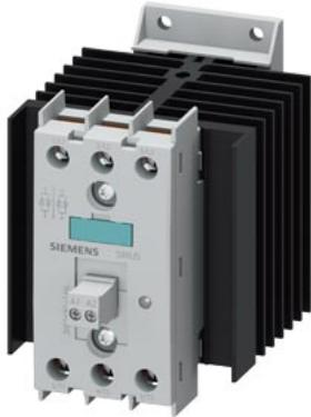
Solid-state contactor 3-phase 3RF2 AC 51 / 30 A / 40 °C 48-600 V / 110 V AC 2-phase controlled screw terminal Blocking voltage 1200 V
