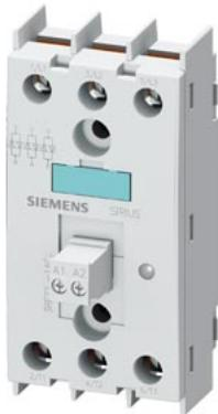
semiconductor relay, 3-phase 3RF2 55 A / 40 °C 48-600 V / 4-30 V DC 3-phase controlled screw terminal blocking voltage 1200 V for mounting on available cooling surfaces
