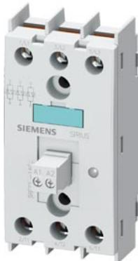
semiconductor relay, 3-phase 3RF2 55 A / 40 °C 48-600 V / 110 V AC 3-phase controlled screw terminal blocking voltage 1200 V for mounting on available cooling surfaces
