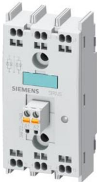
semiconductor relay, 3-phase 3RF2 30 A / 40 °C 48-600 V / 4-30 V DC 2-phase controlled spring-loaded terminal blocking voltage 1200 V for mounting on available cooling surfaces
