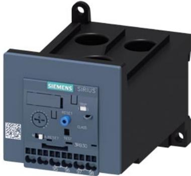
Overload relay 12.5...50 A Electronic For motor protection Size S3, Class 10E
