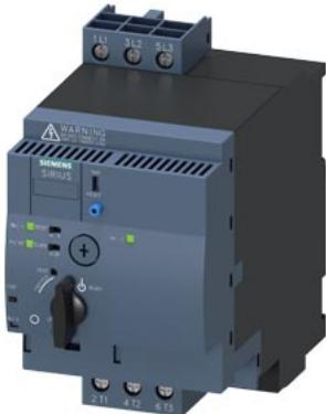
SIRIUS Compact load feeder Reversing starter 690 V 24 V AC/DC 50...60 Hz 3...12 A IP20 Connection main circuit: Screw terminal Connection control circuit: plug-in, without terminals
