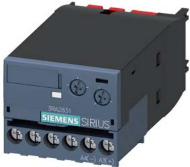
electronic timing relay, ON-delay, with semiconductor output, time range 0.05-100 s, 90-240 V AC/DC, 50/60 Hz, varistor for attenuation of the contactor coils integrated, screw terminal, can be snapped onto the front on contactors 3RT203 / 3RT204
