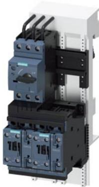
Fuseless motor starter Reversing operation 600VAC Size S0 0.45-0.63A 24V DC screw connection For snapping onto 60 mm busbar systems Type of coordination 2 IQ = 150 KA Also full fills type Of coordination 1 1NO+1NC (per contactor)
