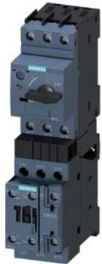
Fuseless motor starter Direct start 600VAC Size S0 1.8-2.5A 110/120VAC 50/60HZ screw connection For screw mounting Or 35 mm rail-mounting Type of coordination 2 IQ = 150 KA Also full fills type Of coordination 1 1NO+1NC (contactor)
