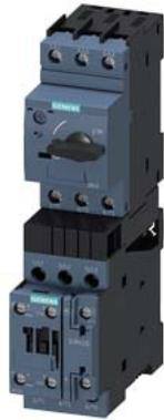
Fuseless motor starter Direct start 600VAC Size S0 0.9-1.25A 24V DC screw connection For screw mounting Or 35 mm rail-mounting Type of coordination 2 IQ = 150 KA Also full fills type Of coordination 1 1NO+1NC (contactor)
