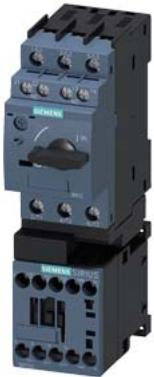
Fuseless motor starter Direct start 600VAC Size S00 0.9-1.25A 220/240VAC 50/60HZ screw connection For screw mounting Or 35 mm rail-mounting Type of coordination 2 IQ = 150 KA Also full fills type Of coordination 1 1NO+1NC (MSP) 1NO (contactor)
