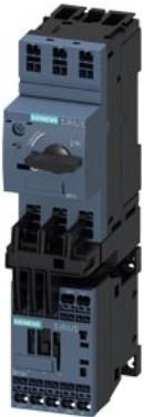
Load feeder fuseless, Direct-on-line starting 400 V AC, Size S00 1.10...1.60 A 24 V DC Spring-type terminal for installation on standard mounting rail (also fulfills type of coordination 1) Type of coordination 2,  $I_q = 150$  kA 1 NO (contactor)
