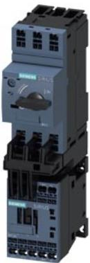
Load feeder fuseless, Direct-on-line starting 400 V AC, Size S00 1.10...1.60 A 230 V AC Spring-type terminal for installation on standard mounting rail (also fulfills type of coordination 1) Type of coordination 2,  $I_q = 150$  kA 1 NO (contactor)
