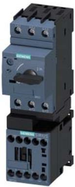
Load feeder fuseless, Direct-on-line starting 400 V AC, Size S00 0.45...0.63 A 230 V AC screw terminal for installation on standard mounting rail (also fulfills type of coordination 1) Type of coordination 2,  $I_q = 150 \text{ kA}$  1 NO (contactor)
