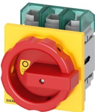
SENTRON 3LD5 switch disconnector UL, EMERGENCY-OFF switch, 3-pole, approved according to UL 489, UL 60947-4-1 and IEC 60947-3, UL: 60 A, SCCR 50 kA at 480 V AC, operational power @ 480 V AC 3-phase: 40 hp, IEC: 63 A, operational power at AC-23 A at 400 V: 30 kW, front-mounted, rotary operating mechanism, red/yellow, 4-hole mounting of the handle, including terminal covers for the infeed side
